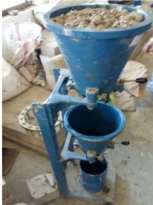
Fig. – 3 Compaction Factor Test
