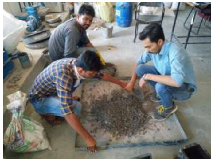
Fig. - 1 Mixing of Alkaline solution with Fly Ash and Aggregates
