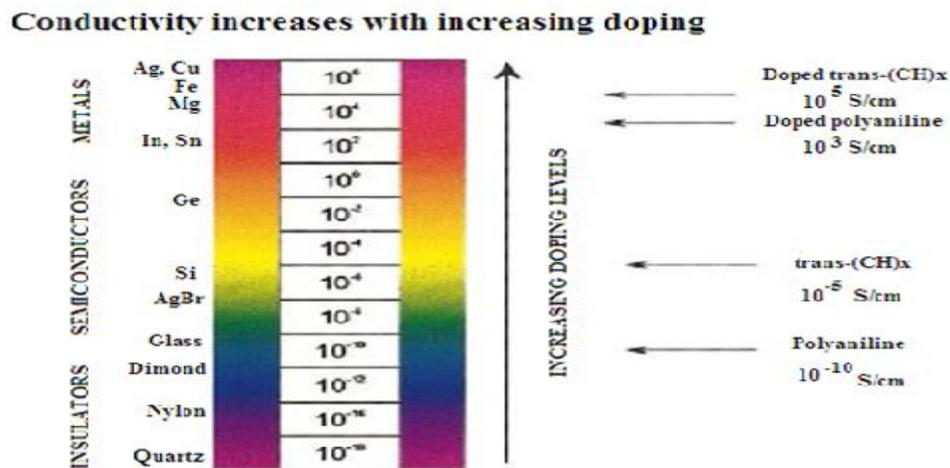
Figure2. Conductivity comparison between conjugated conducting macromolecules (Polymers) and other materials
