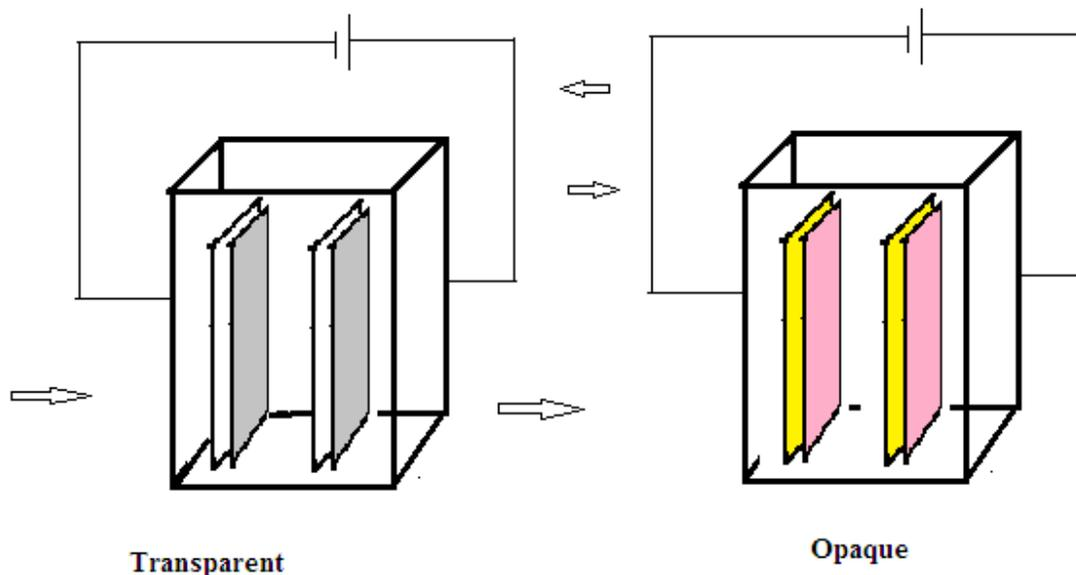
**Figure 4: Electrochromic window operation**
