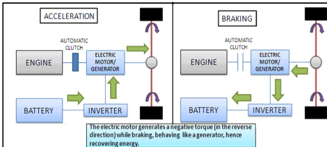
Fig.2. Regenerative Braking System.
