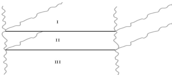
A dielectric slab waveguide consists of three dielectric layers with different refractive indices. Practical rectangular-geometry optical waveguides are most easily understood as variants of the simple dielectric slab waveguide, also called planar waveguide. The slab waveguide consists of three layers of materials with different dielectric constants, extending infinitely in the directions parallel to their interfaces.
