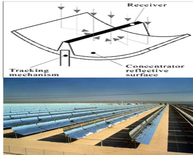
Figure:- Parabolic trough system
