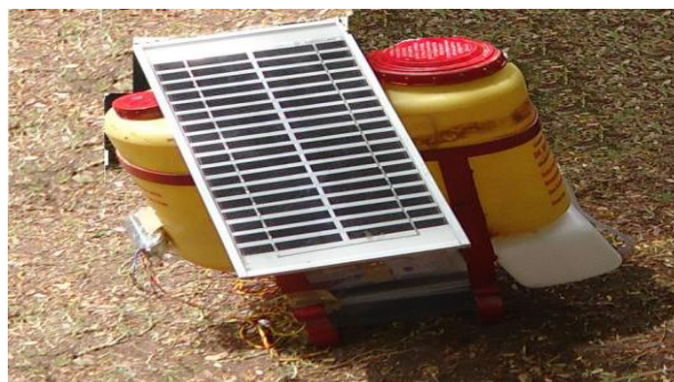
Fig. 1. Solar Operated Spraying
