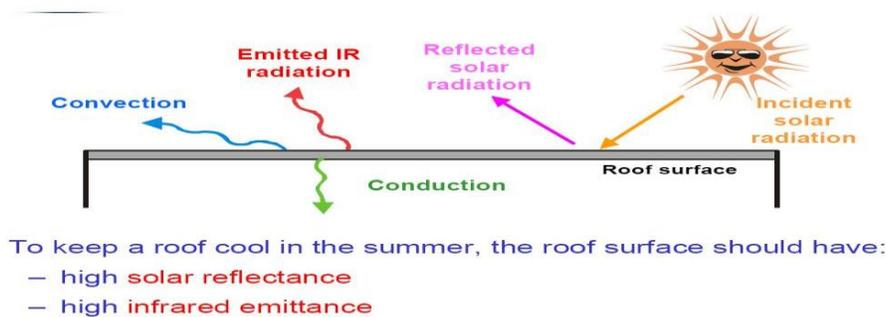
Fig . Working of green roof
