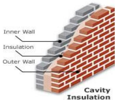
Fig. Shows the system of cavity wall
