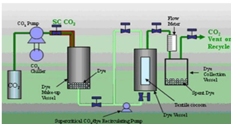
Fig: 2 CO<sub>2</sub> dyeing of PET
