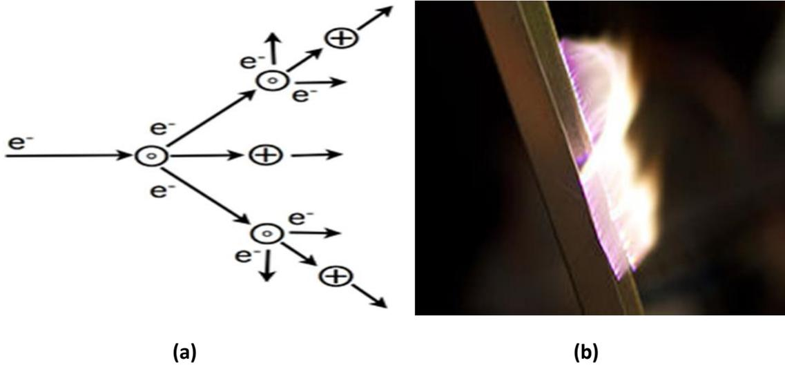
Fig:4 (a) Cascade process of ionization. Electrons are 'e-', neutral atoms 'o', and cations '+',
