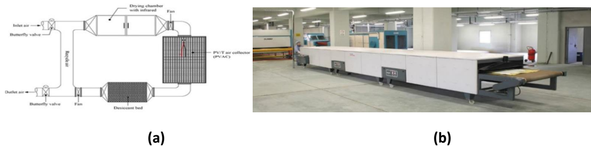
Fig:5 (a) Principle of IR generation, (b) IR dryer.
