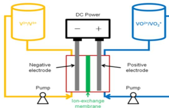
Fig 3: Vanadium Redox Flow Battery
