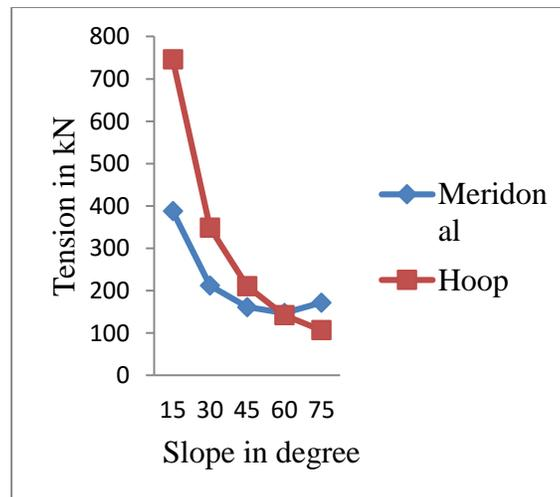
Figure 5 Comparison of meridional and hoop tension
