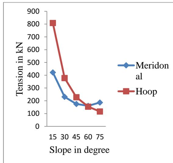
Figure 6 Comparison of meridional and hoop tension
