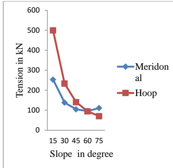
Figure 4 Comparison of meridional and hoop tension
