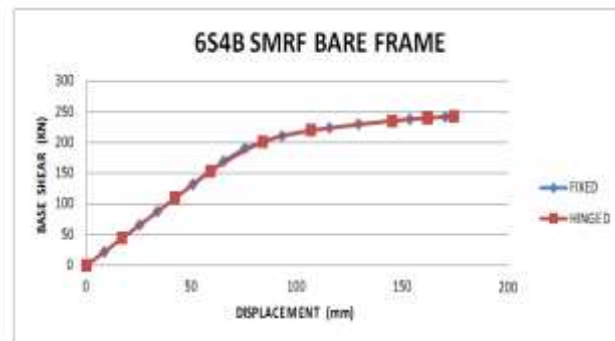
Figure shows the pushover curves of 6S4B SMRF with both fixed and hinged support condition and no infill.
