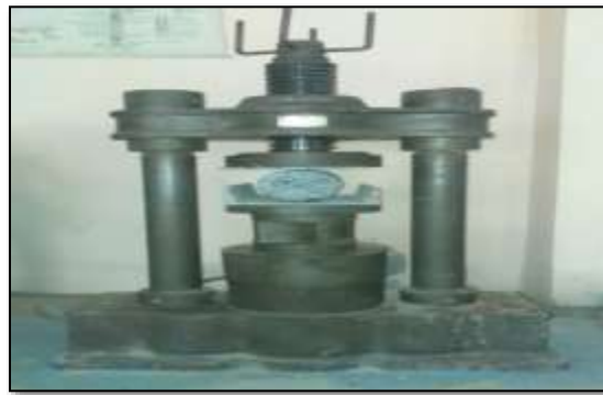
Fig. 4: Split Tensile Strength Test
