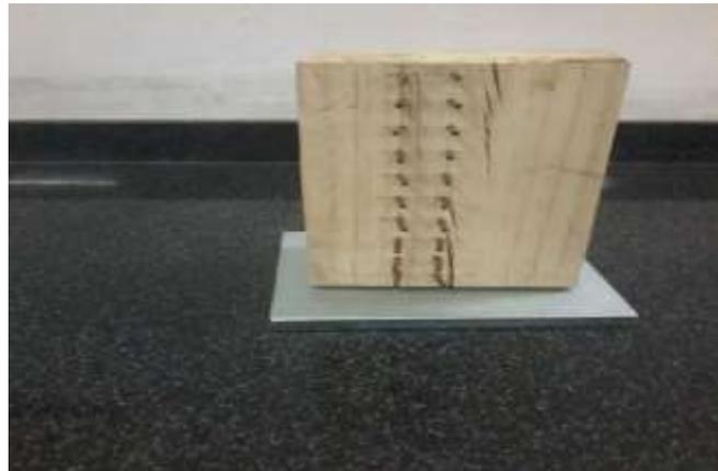
**Figure 3: Building Model with pressure tappings**
