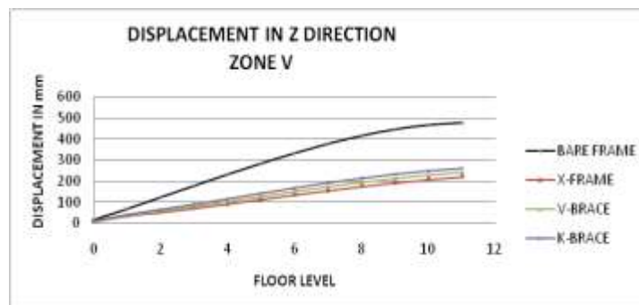
Fig 13: Lateral Displacements (mm) in Z direction
