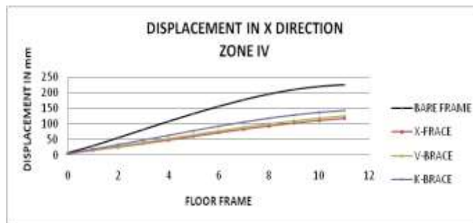
Fig 8: Lateral Displacements (mm) in X direction
