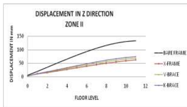
Fig 10: Lateral Displacements (mm) in Z direction
