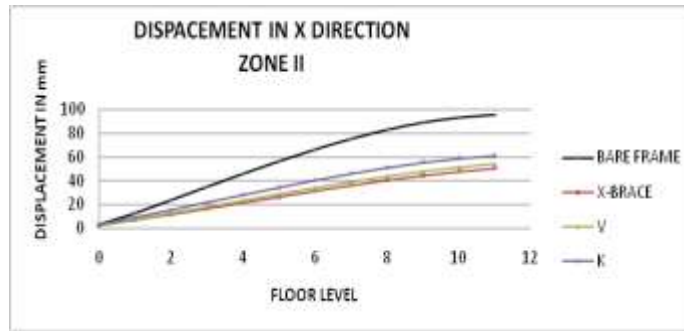
Fig 6: Lateral Displacements (mm) in X direction
