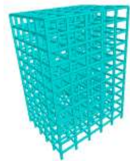
Fig 2: Structure frame without Bracing system
