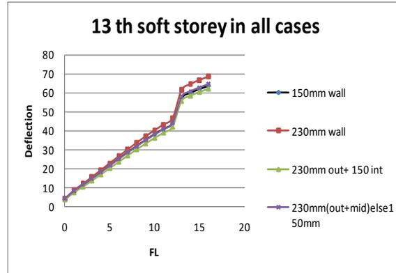
Graph for irregular structure for various infill wall cases with different level soft storey as below.
