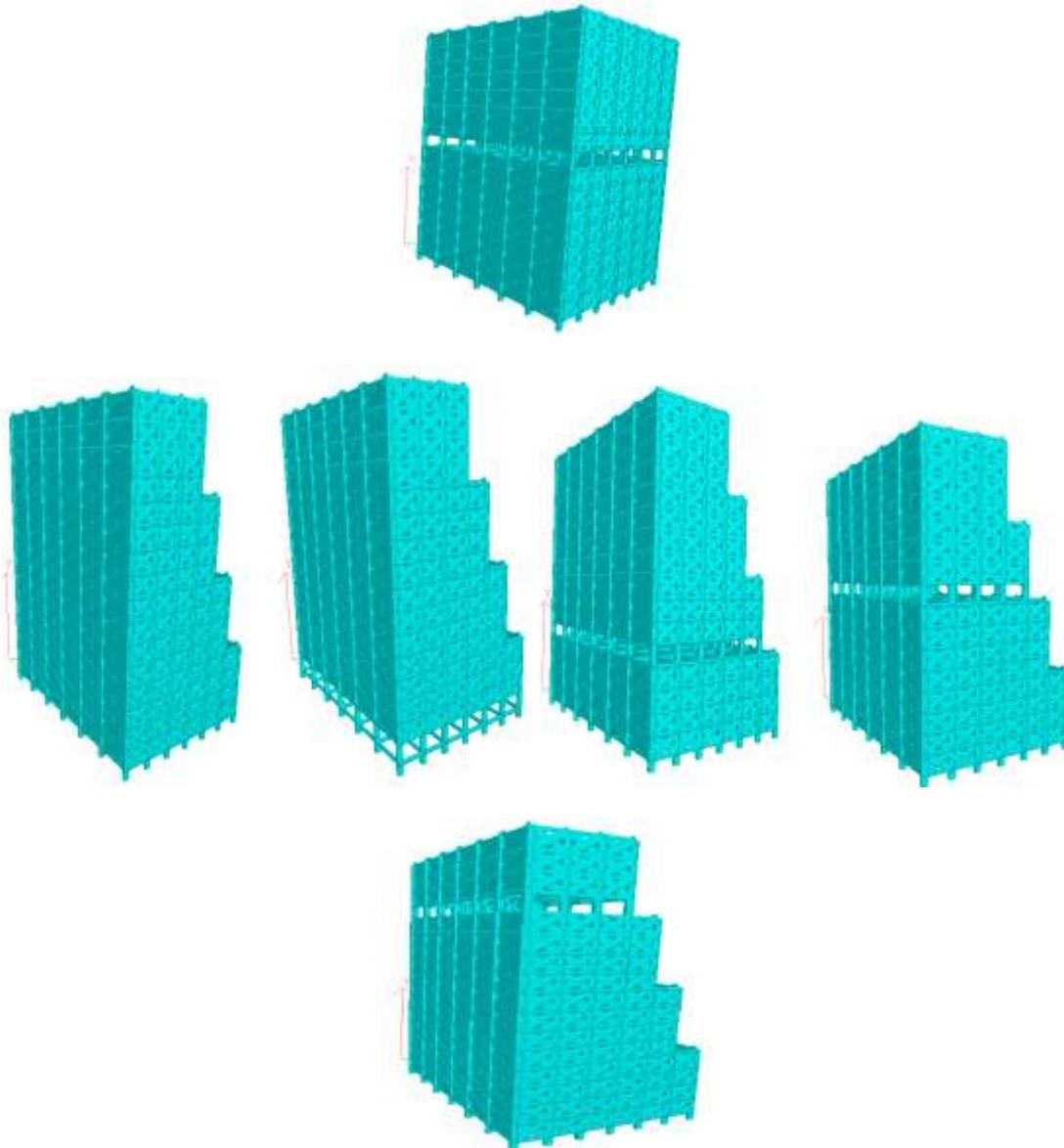
**Figure Shows different types modeling of structure for regular and irregular buildings at ground soft storey, 5<sup>th</sup> soft storey, 9<sup>th</sup> soft storey and 13<sup>th</sup> soft storey**
