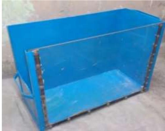
**Figure 2 Test Tank**
