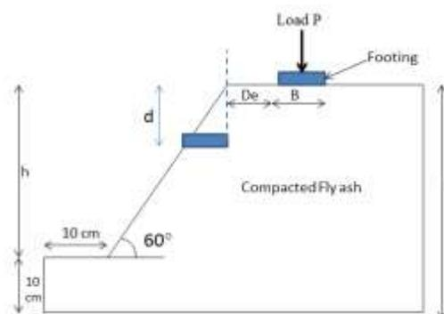
Figure 7: Schematic view of test configuration
