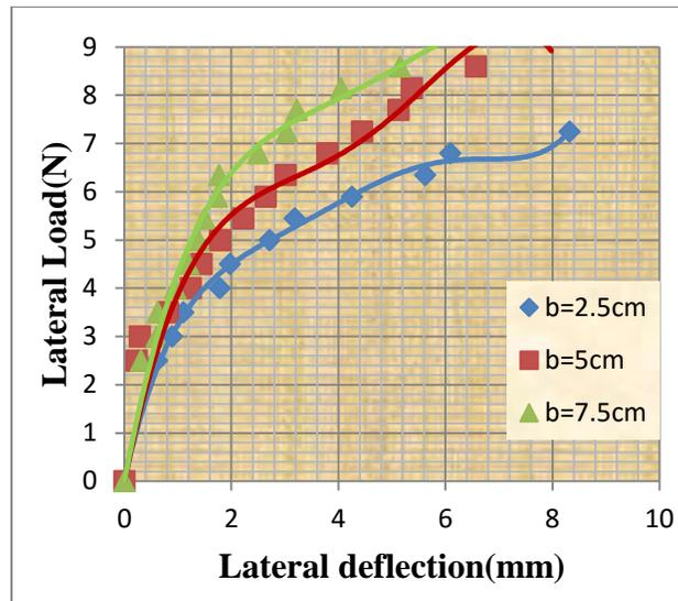
Figure 5: Lateral Load vs Lateral deflection of short pile for 30° of inclination
