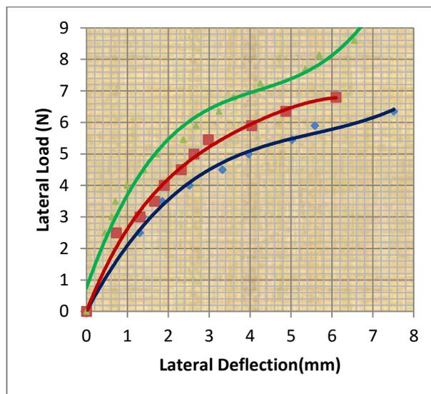
Figure 4: Lateral Load vs Lateral deflection of short pile for 15° of inclination
