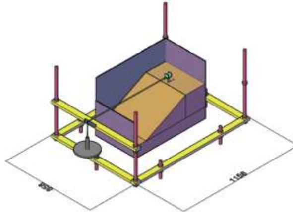
**Figure 2: 3D View of Test Tank**
