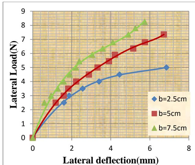
Figure 3: Lateral Load vs Lateral deflection of short pile for 0° of inclination
