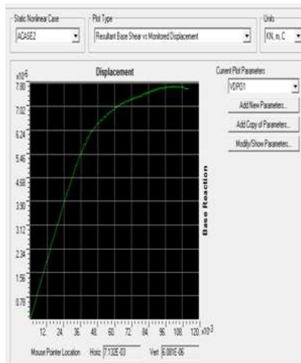
Figure 3: Push over curve
