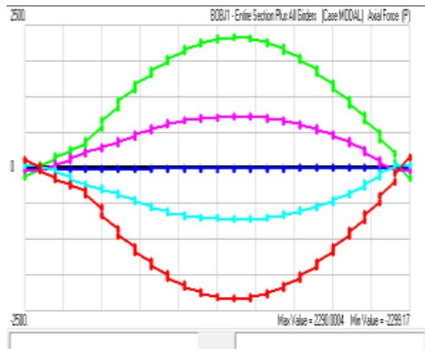
Figure 7: Variation of Axial Force for Entire Section and All Girders
