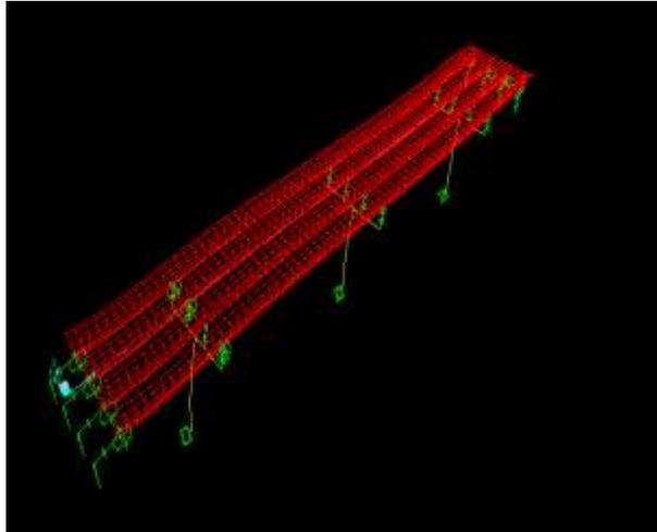
Figure 2: Deformed Shape Corresponding to EQ X
