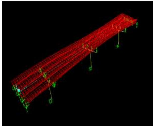
Figure 3: Deformed Shape Corresponding to EQ Y
