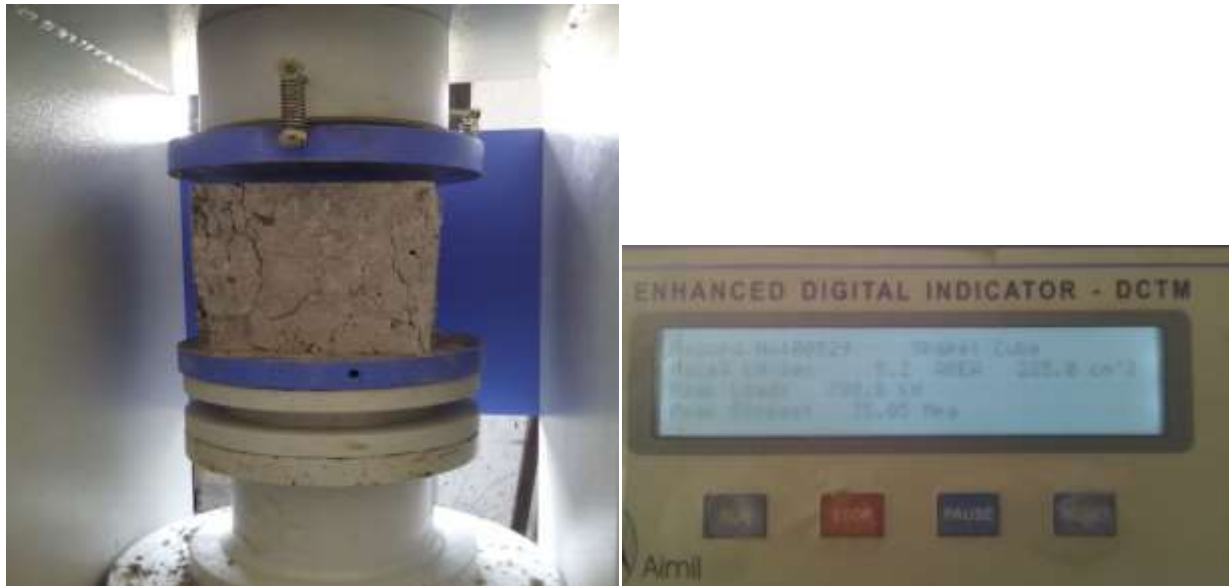
Step 4: testing of compressive strength of the cube using CTM
