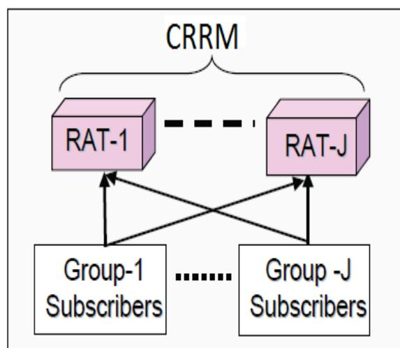
**Fig. 2. Common RRM in heterogeneous wireless networks**
