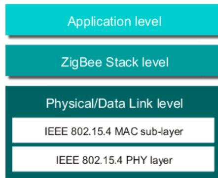
**Figure 1: Zigbee protocol stack**
