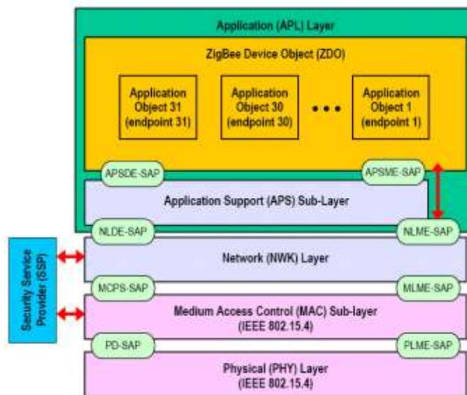
Figure 2. Layered architecture of Zigbee
