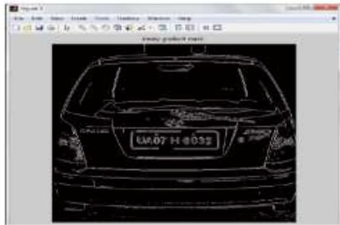
**Fig.5. Binary gradient image with sobel edge detector.**
