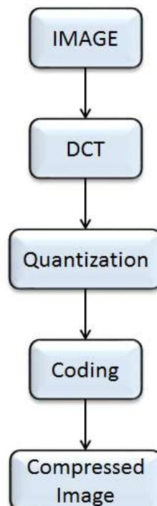
Figure 2: Block Diagram of JPEG Image Compression
