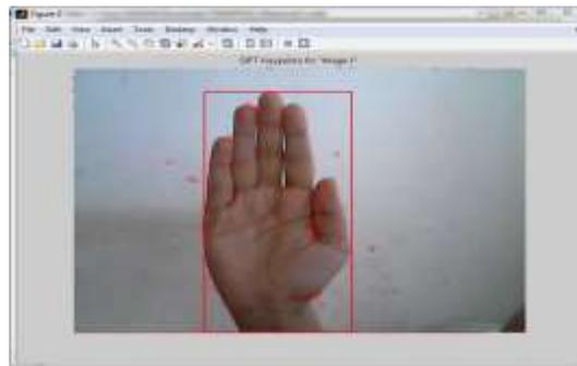
**Figure 7. The real time SIFT feature of hand gesture**
