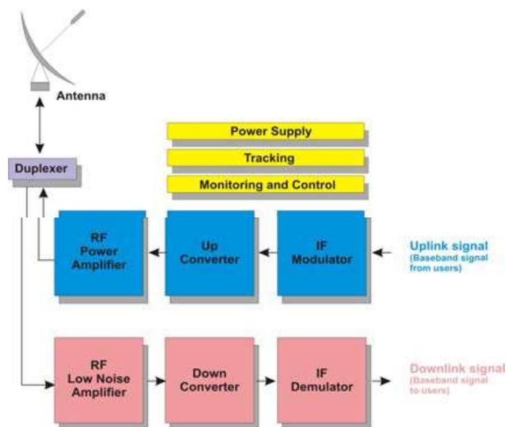
Fig. 1. The satellite ground station architecture
