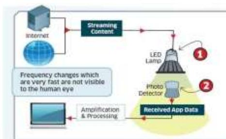
Fig. 4. Block diagram of Li-Fi system [6]
