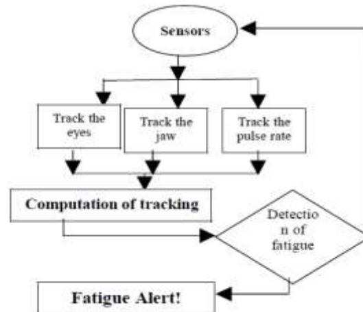
**Figure 3: Flowchart for process of fatigue detection system**
