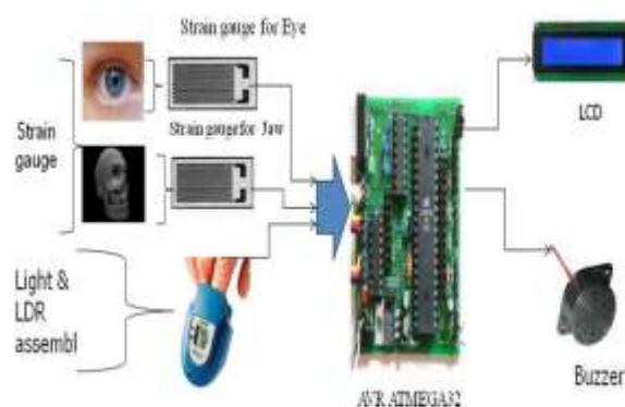
Fig1. Proposed Fatigue detection system
