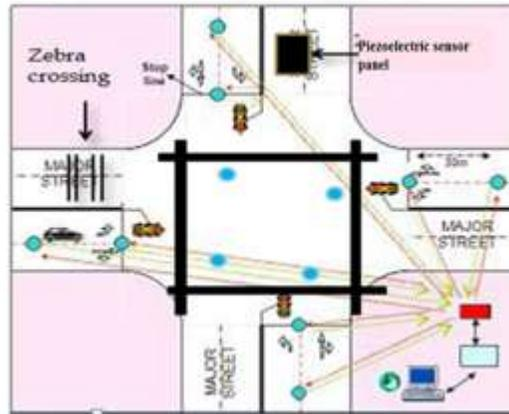
**Fig (1): Automatic traffic control density**
