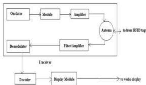
**Fig (2) Block Diagram for RFID**
