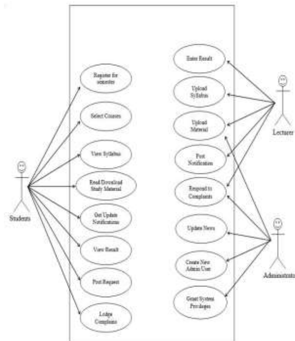
Fig. Use case diagram of student portal
