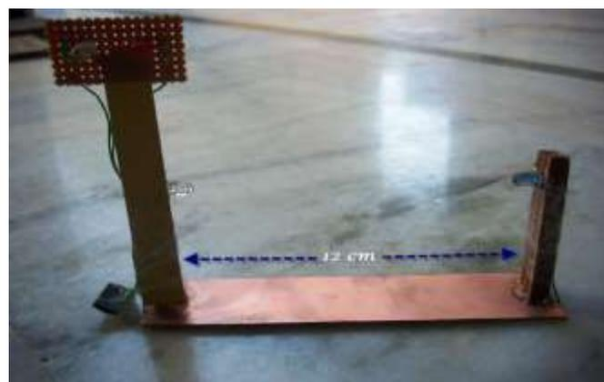
Fig (4): Approximate distance between two sensors
