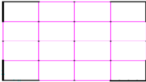
Fig. 2 MR TYPE 1 (Model of Building with Shear Wall type1 at corner)
