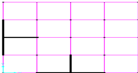
Fig. 6 MIR TYPE 5 (Model of Irregular Building with Shear Wall present irregularly)
