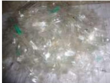
**Fig. 3.1 : Polyethylene Terephthalate (PET) Fibers**
