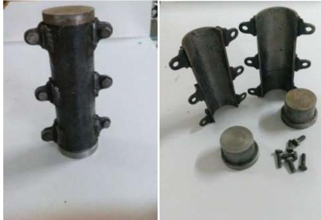
Fig. 3.2 : Cylindrical mould (50 mm x 100 mm)
