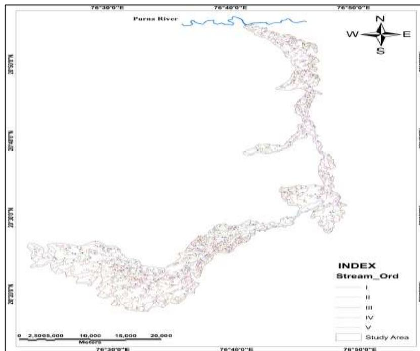
Fig. 2 Drainage map with stream order of the Man River Basin
