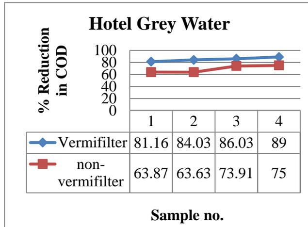
Figure 7% Reduction in COD of HOTEL greywater with vermifilter and non-vermifilter
