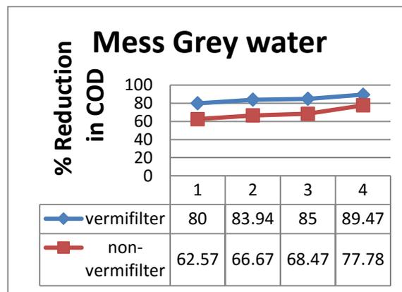
Figure 7% Reduction in COD of MESS greywater with vermifilter and non-vermifilter.
