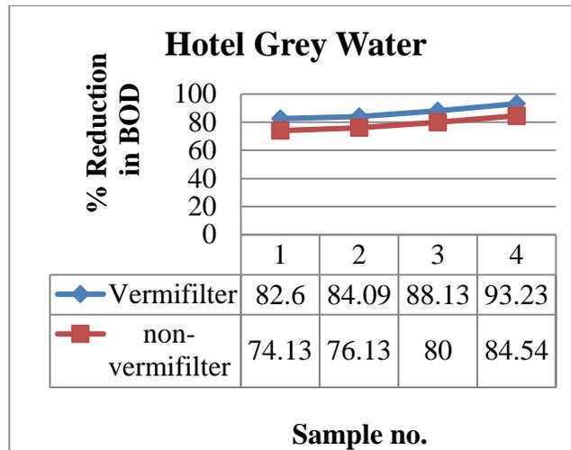
Figure 6% Reduction in BOD of hotel greywater with vermifilter and non-vermifilter.
