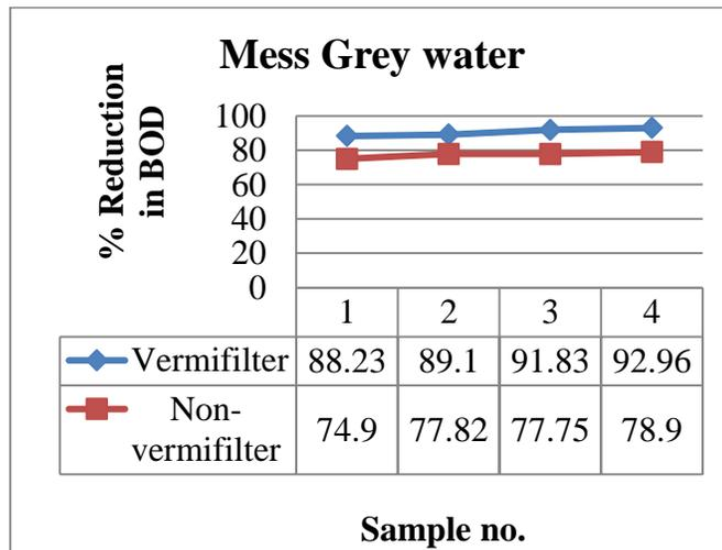
**Figure 5%** Reduction in BOD of mess greywater with vermifilter and non-vermifilter.
