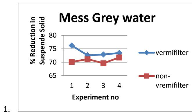
Figure 3% Reduction in Suspended solid of mess greywater with vermifilter and non-vermifilter.
