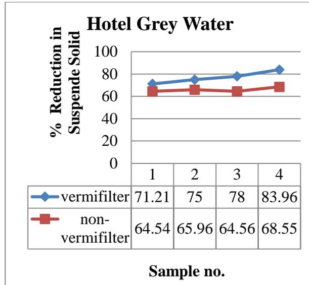
**Figure 4%** Reduction in suspended solid of hotel greywater with vermifilter and non-vermifilter.
