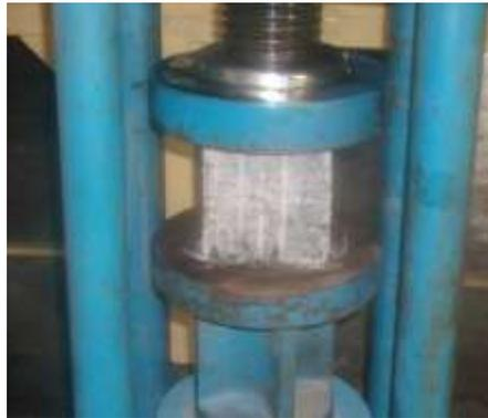
Fig. 1.6 “Testing of compressive strength test specimen
