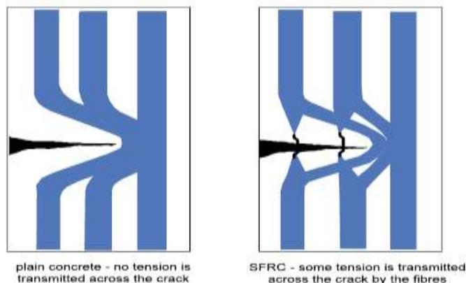
**Fig 1.1: Stress Lines in concrete Under Tension**
