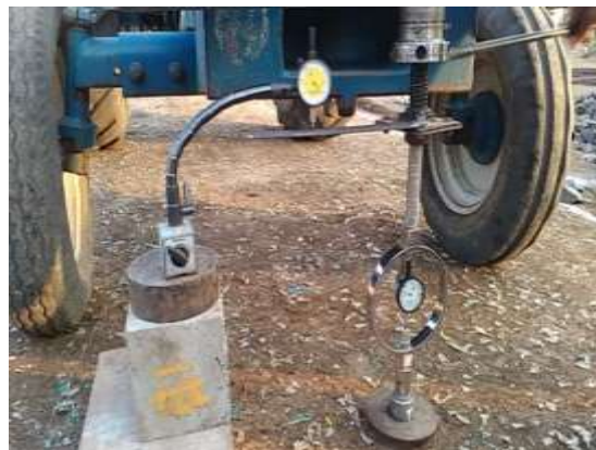
Figure 7. Typical Setup for Unsoaked Field CBR on Composite Subgrade of Model Flexible Pavement
