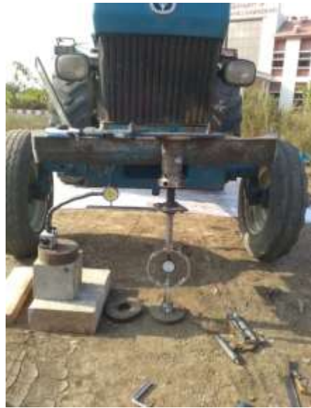
Figure 6. Typical Setup for Unsoaked Field CBR on Artificial Subgrade of Model Flexible Pavement
