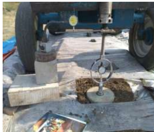
Figure 9. Performed Soaked Field Tests on Artificial and Composite Subgrade
