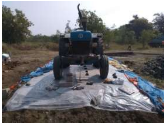
Figure 8. Arrangement for Soaked Field CBR Test
