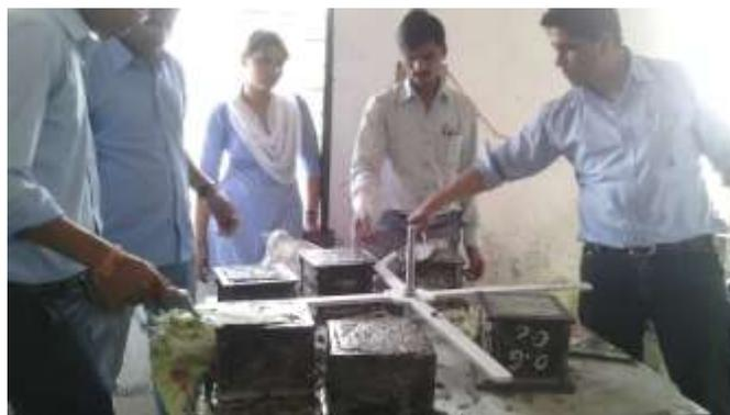
**Figure 1 Concrete cube casting**
