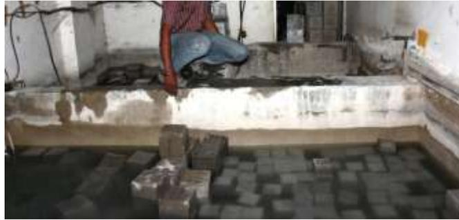
Figure 2 Curing of concrete cubes for 7 days and 28 days
