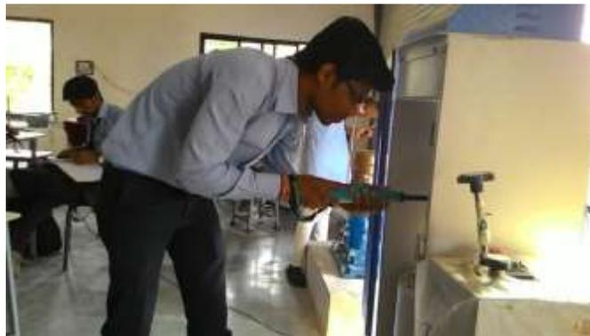
Figure 4 NDT by using Schmidt rebound hammer
