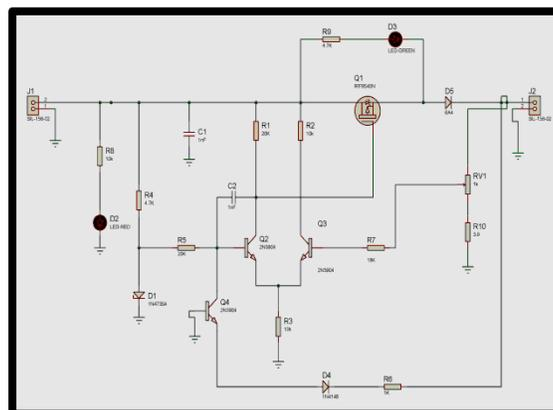
Fig 2.1.2: Circuit Diagram of MPPT on Proteus
