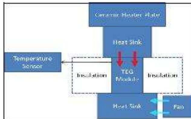
Figure 3: Overview of Experimental Setup
