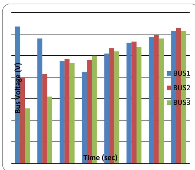
Figure 3: Bus voltages without STATCOM
