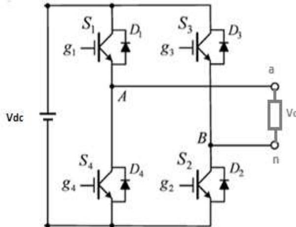
Figure.1 - Single Phase H-bridge Inverter.
