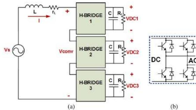
Figure 2:(a) Schematic diagram of a 7-level CHB in active rectifier configuration, and (b) a single HB circuit.
