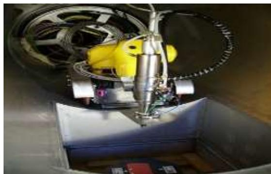
**Figure 6 -Charli will be used for pipe-cutting work at Superphenix [3]**
