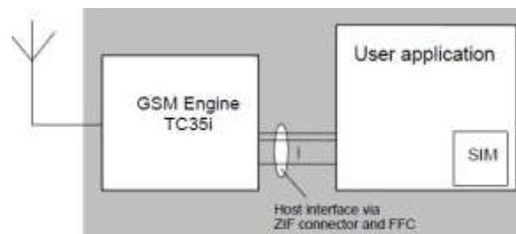
**Fig 3. BLOCK DIAGRAM OF A CELLULAR APPLICATION**
