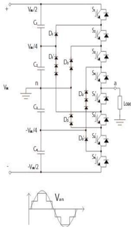
Fig.1 One phase-leg for a two-level NPC Inverter
