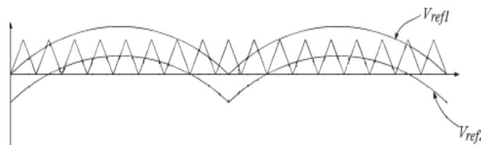
Figure 3. PWM switching signal generation for 5-level multilevel inverter.
