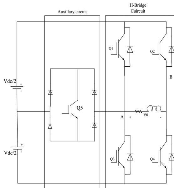
Figure 2. Topology of 5-level multilevel inverter.
