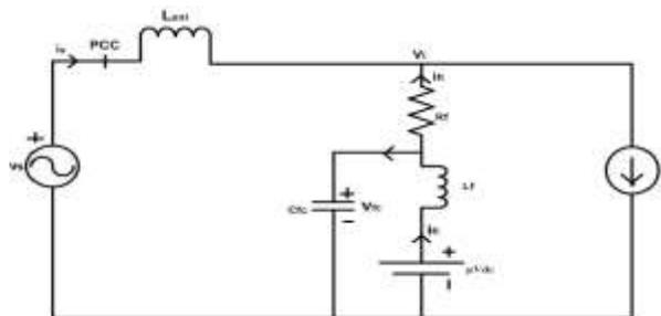
Fig.1 – Single-phase equivalent circuit of DSTATCOM in a distribution network.
