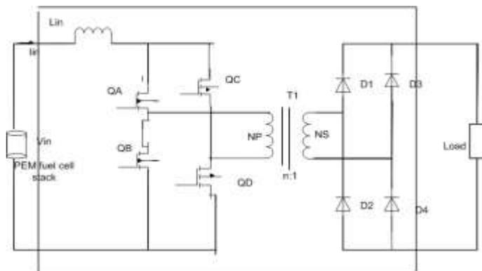
Fig.1 – PEM fuel-cell power converter system
