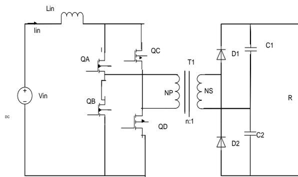
Fig.3- Current-fed full-bridge dc-dc converter
