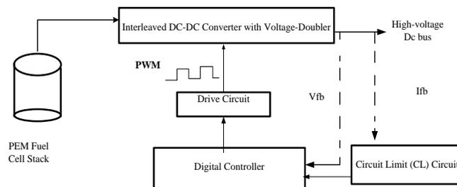
Fig.2 Digital-controlled interleaved dc-dc converter
