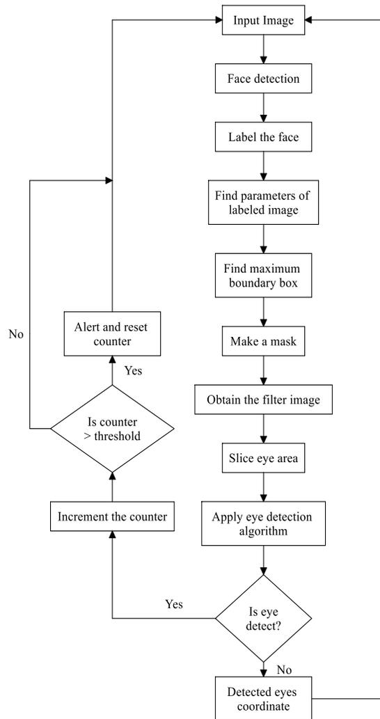
Figure 3:- Proposed detailed data flow diagram for Monitoring and Prediction of Driver Fatigue.
