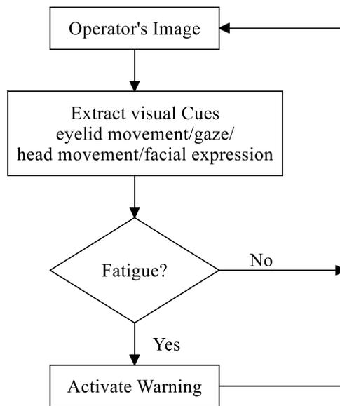
**Figure 1:- Basic flowchart of the proposed system for Monitoring and Prediction of Driver Fatigue**
