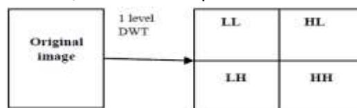
Fig. 2. Single Level DWT Decomposition of Image.
