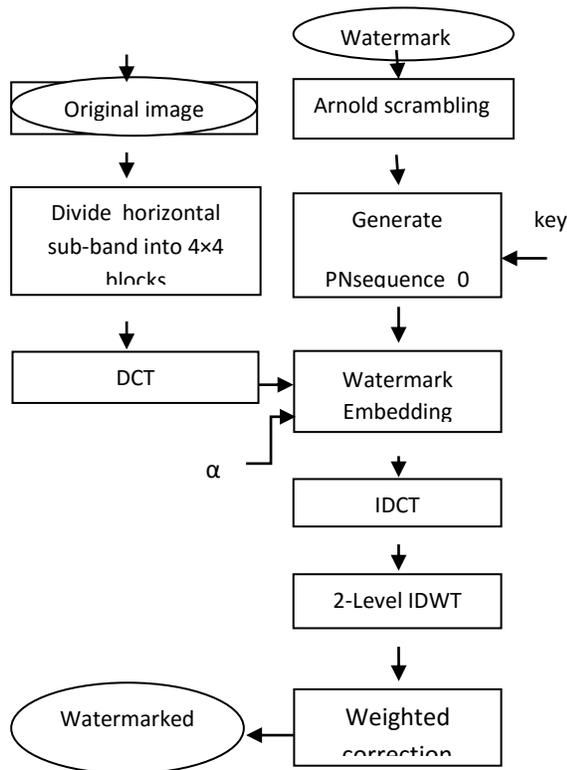
**Fig. 4. Embedding of watermark bits into the host image.**
