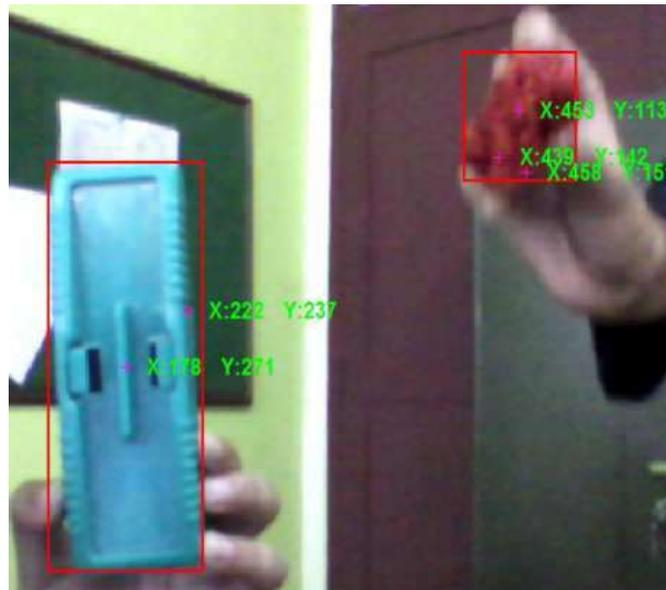
Fig 4:Tracking using Kalman Filter
